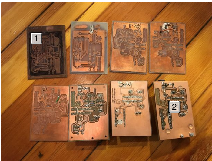
1. first etch didn't go so well, but I quickly got the hang of it on the 2nd attempt. You can see I went through a few iterations until I got to the final version. Best part about doing this at home is that it's FAST - you can make a board in about an hour, so tweaking your design is pretty easy. 2. the final board!
